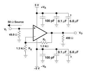
Figure 33. Wideband, Noninverting Gain Configuration
