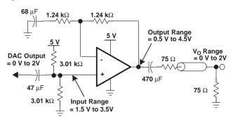
Figure 42. AC-Coupled Wide Output Swing Single-Supply Video Amplifier
