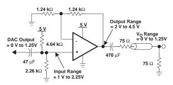
Figure 41. AC-Coupled Input and Output Single-Supply Video Amplifier
