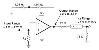
Figure 38. DC-Coupled Single-Supply Video Amplifier
