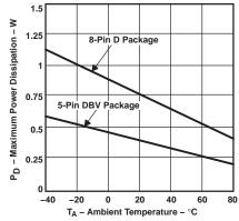
$\theta_{JA}$  = 170°C/W for 8-Pin SOIC (D)  $\theta_{JA}$  = 324.1°C/W for 5-Pin SOT-23 (DBV)  $T_{J}$  = 150°C, No Airflow
