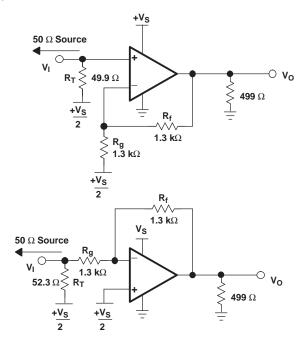
Figure 35. DC-Coupled Single Supply Operation
