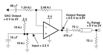
Figure 44. Inverting AC-Coupled Wide Output Swing Single-Supply Video Amplifier
