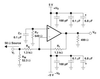
Figure 34. Wideband, Inverting Gain Configuration
