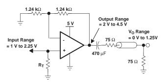
Figure 39. AC-Coupled Output Single-Supply Video Amplifier
